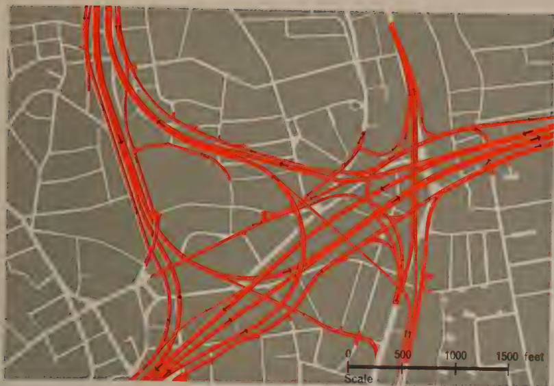
242 An interchange planned for the Inner Loop at Boston. It occupies about 100 acres. Compared with this, the interchanges shown in the examples worked out in Chapter III seem quite modest, yet they may be as much as British cities can stand of this space-taking engineering.
